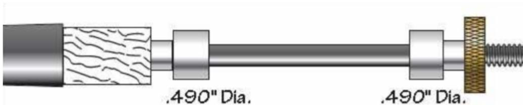
1. Assemble the bushings and blank on the razor mandrel as shown below.
